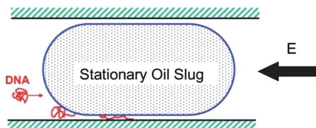
**Fig. 9** Deformation of a DNA molecule that is electrokinetically driven into confinement between a stationary oil “slug” and microchannel wall. Reprinted figure with permission from S.-F. Hsieh and H.-H. Wei, *Phys. Rev. E: Stat., Nonlinear, Soft Matter Phys.*, 2009, **79**, 021901. Copyright (2009) by The American Physical Society.
