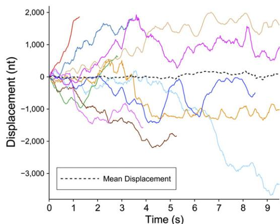
**Fig. 3.** Single-molecule position trajectories of several SSBs at 4.1 pN tension. The position trajectories of different SSBs are drawn in continuous lines of different colors. A black broken curve represents the mean displacement of all trajectories. The displacement was measured in nanometers and then converted into number of nucleotides by using the extension per nucleotide at the corresponding force (Fig. S2b).
