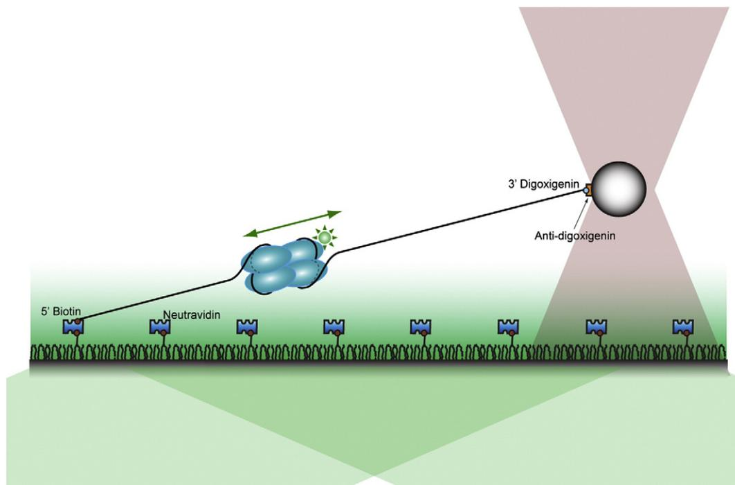
**Fig. 1.** Schematic of the experimental setup. One end of an ssDNA construct is immobilized on a polyethylene-glycol-coated surface, and the other end is attached to a polystyrene bead confined in the optical trap (pink gray). A green excitation laser selectively illuminates molecules within a few hundred nanometers from the coverslip surface by total internal reflection.
