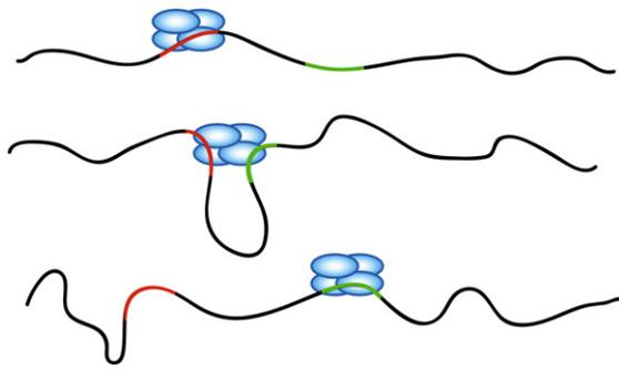
**Fig. 6.** Schematic depicting the concept of intersegment transfer. In this model, SSB migrates from one location to the other via a long-range intersegment transfer. An SSB is bound at a location (red) on a long ssDNA. When the other segment (green) of the same strand on which the SSB is bound makes contact with the SSB via random fluctuations, the SSB then transfers to the new location.
